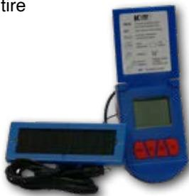
The Baccara controller (above) is fully independent, whereas the QTech controller (right) can be updated from a distance. The QTech uses a sophisticated mesh network which enables updates over difficult terrain to all G-Set units from a single location.
