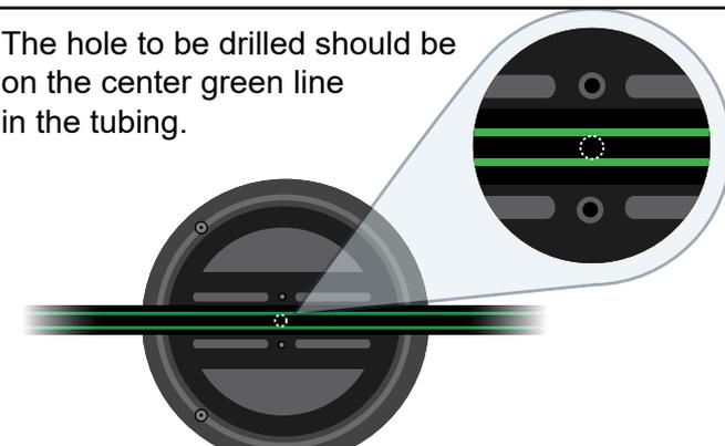
**C** Drill a 14mm hole in the tubing at the desired spacing.
