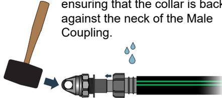
③ Hand tighten the collar of the Male Coupling onto the tubing, then finish by using a combination of pipe wrenches and channel locks to securely tighten the collar. This causes the barbs to bite into the interior and exterior of the K.PIPE® tubing for a strong connection.
