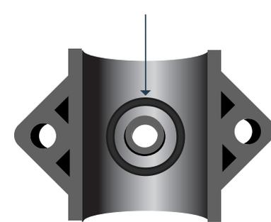
**G** Push the K-LINE® tapping saddle down over the threaded posts and be certain that the nipple on the underside of the tapping saddle is inserted into the 14mm hole.
