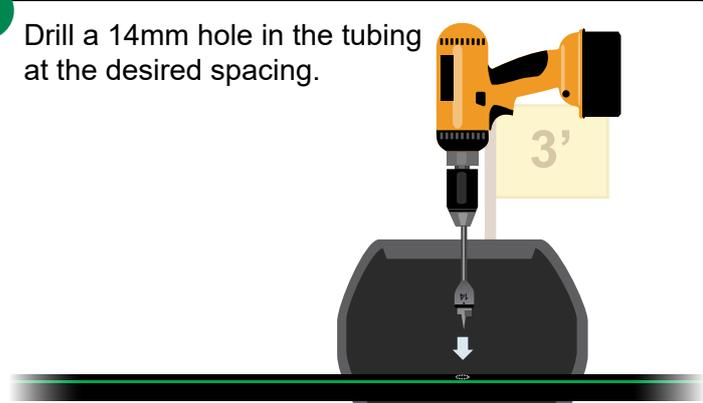
**D** **Caution: Do not use a 3rd party drill bit.** The K-LINE® Bit has a limiter attached to it to prevent the bit from being inserted too deeply and puncturing the opposite tubing wall.
