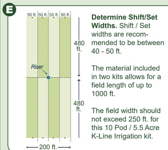
K-Line's adaptability is increased when 2 kits are combined. The example layout in this manual allows 2 Kits to be combined to irrigate a 4.4 acre area, but K-Line's almost limitless flexibility allows you an even greater range of options – from irrigating larger areas with a single 10 sprinkler/pod K-Line, to making two K-Lines of different lengths to irrigate several different sized areas.
