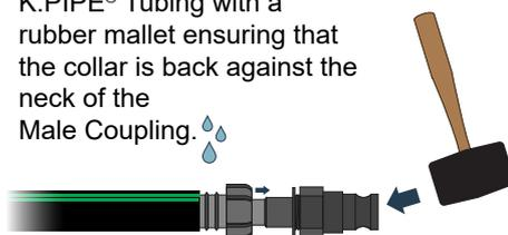
③ Hand tighten the collar of the Male Coupler onto the tubing, then finish by using a combination of pipe wrenches and channel locks to securely tighten the collar. This causes the barbs to bite into the interior and exterior of the K.PIPE® tubing for a strong connection.
