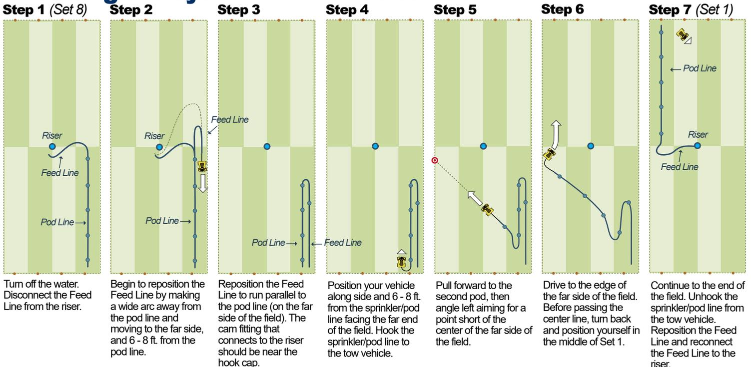
Turn off the water. Disconnect the Feed Line from the riser.
