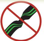
**DO NOT ALLOW IT TO TWIST!** The green line(s) should face up for the entire length of the tubing. Do not make the end cut until the pods have all been installed.
