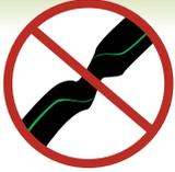
**DO NOT ALLOW IT TO TWIST!** The green line(s) should face up for the entire length of the tubing.
