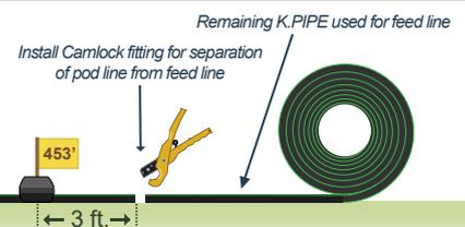
Use  $1\frac{1}{2}$ " or 2" Poly Pipe cutters or a Hacksaw to make a square cut at the end of the Pod Line 3 - 5 ft. past the final marker. Make sure that the cut end is square and that any burrs are removed. **RESUME INSTRUCTIONS ON PAGE 5, STEP 8.**
